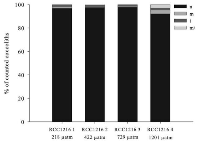
**Figure 6** Percentage of normal (n), malformed (m), incomplete (i), malformed and incomplete (m/i) coccoliths (strain RCC1216) vs. CO<sub>2</sub> partial pressure. Values represent an average of triplicate experiments. CO<sub>2</sub> partial pressures were taken from (Langer et al., 2009).
